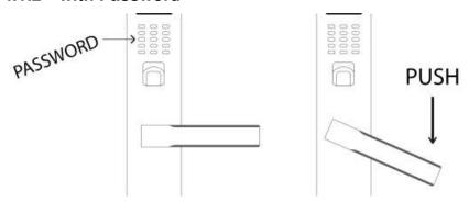
Enter password & press ENTER to unlock the door. Push the handle.
