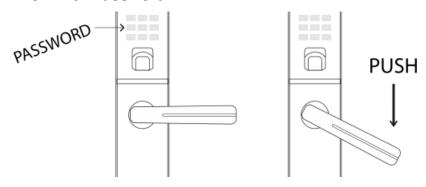
Enter password & press **ENTER** to unlock the door. Push the handle.
