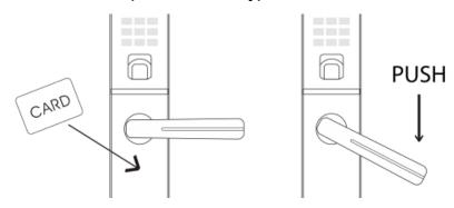
Scan card to unlock the door. Push the handle.
