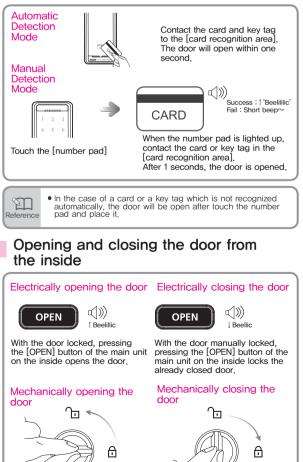
With the door locked, turn the manual switchgear to 1 direction.
