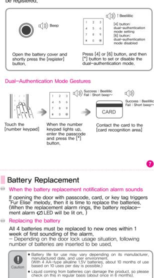
After the battery replacement notification alarm is sounded, pass code/card registration, changes, or feature setting cannot be made until the batteries are replaced.
