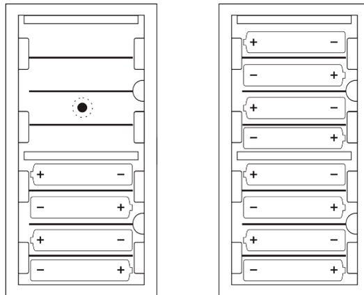
One set of 4 AA batteries or two sets of 4 AA batteries are required to power the lock.
