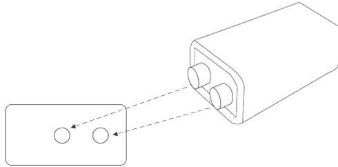
Just plug a 9V battery on the 2 pins located below the front panel and you can operate your lock as usual. Don't forget to change your batteries afterward.
