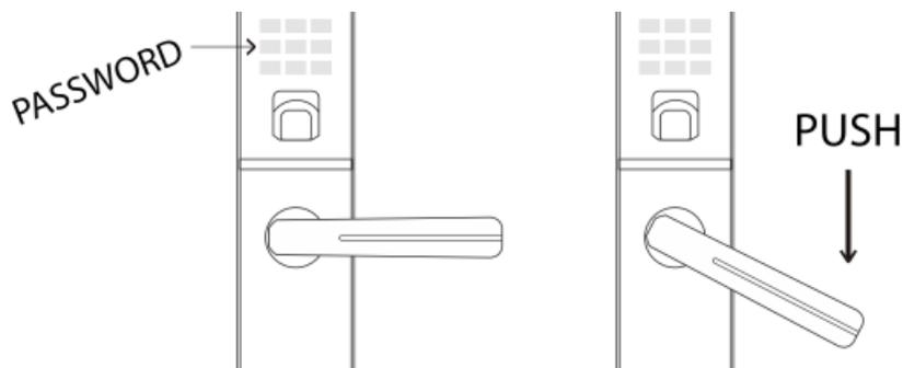
Enter password & press **ENTER** to unlock the door. Push the handle.
