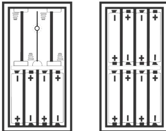
One set of 4 AA batteries or two sets of 4 AA batteries are required to power the lock.
