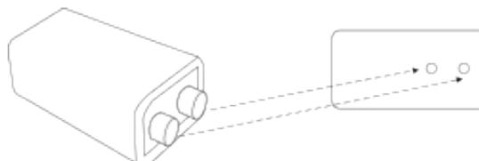
Just plug a 9V battery on the 2 pins located below the front panel and you can operate your lock as usual. Don't forget to change your batteries afterward.
